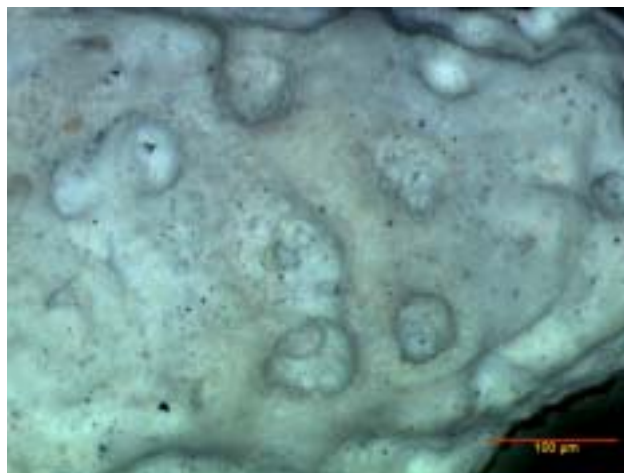
Figure 3. Optical Photograph of SCT02-098 Particle. Black particles are magnetite
