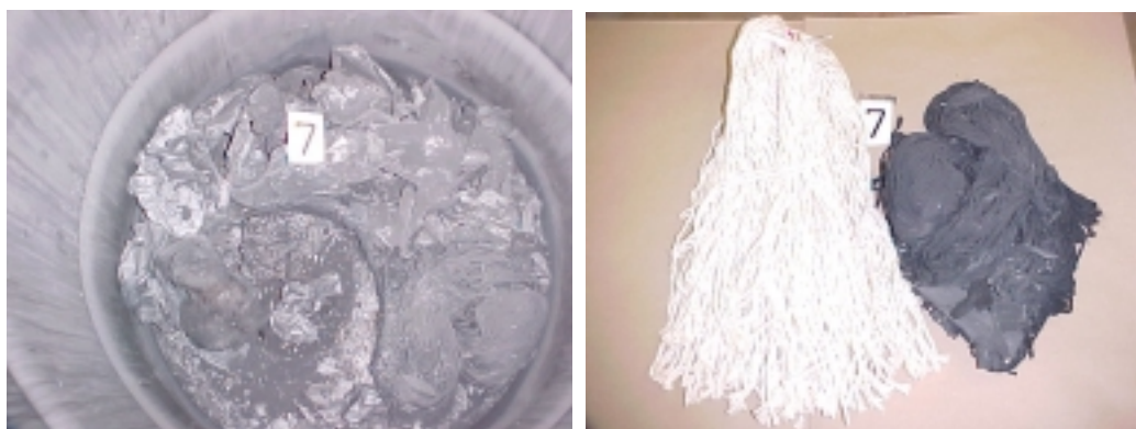
Figure 49. The Remains of the Paper and Mop Heads Pyrolyzed in Drum #7 Figure 50. A Pyrolyzed Mop Head from Drum #7 Compared to an Untreated Mop Head
