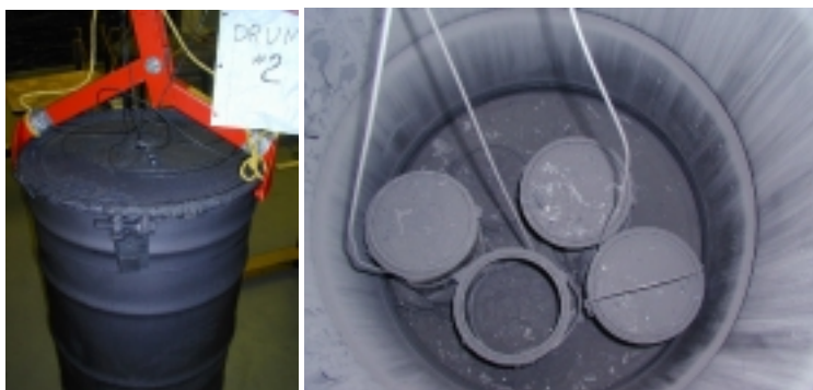
Figure 14. Drum #2 Following Pyrolysis Figure 15. The Interior of Drum #2 Following Pyrolysis
