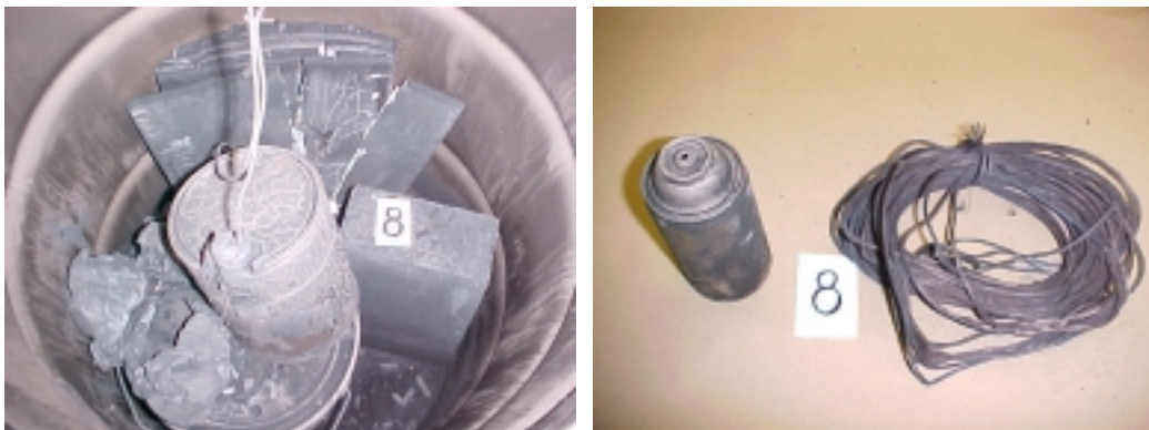
Figure 54. The Interior of Drum #8 Following Pyrolysis
