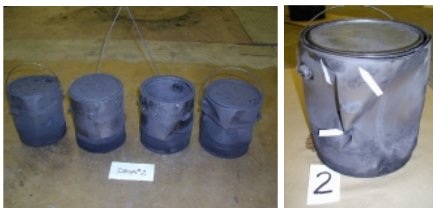
Figure 16. The Contents of Drum #2 Following Pyrolysis Figure 17. Paint Can from Drum #2 After Pyrolysis. Arrows indicate Leak Points
