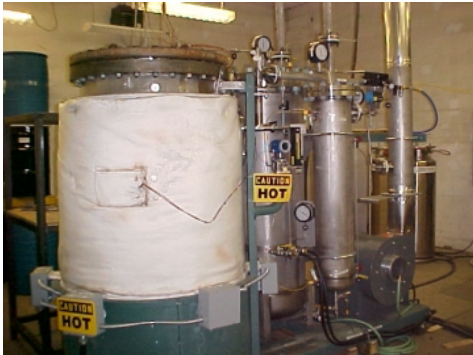
Figure 2. The THOR SM Drum Pyrolysis Test System Fully Assembled and Ready for Operation
