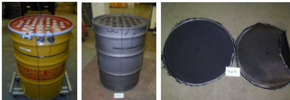
Figure 8. Drum #1 Ready for Pyrolysis
