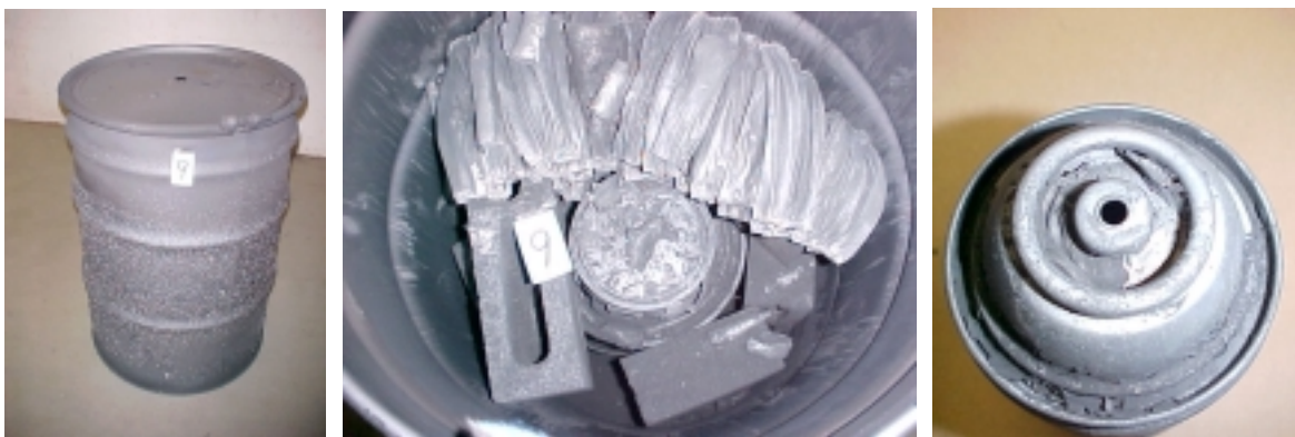
Figure 60. Drum #9 Inner 55-Gallon Drum Following Pyrolysis
