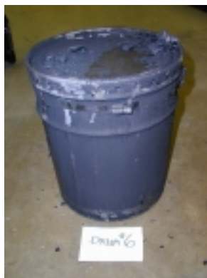
Figure 39. 5-Gallon Can from Drum #6 Following Pyrolysis
