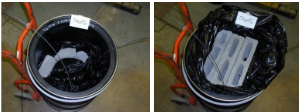
Figure 34. Contents of Lower Half of Drum #6 Prior to Pyrolysis.
