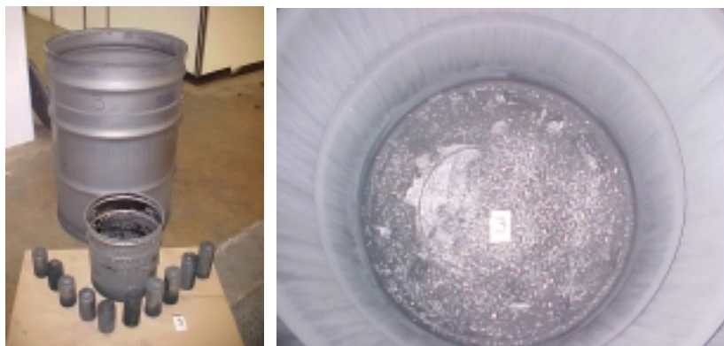
Figure 21. The Contents of Drum #3 Following Pyrolysis
