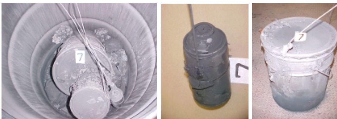
Figure 44. The Interior of Drum #7 Following Pyrolysis
