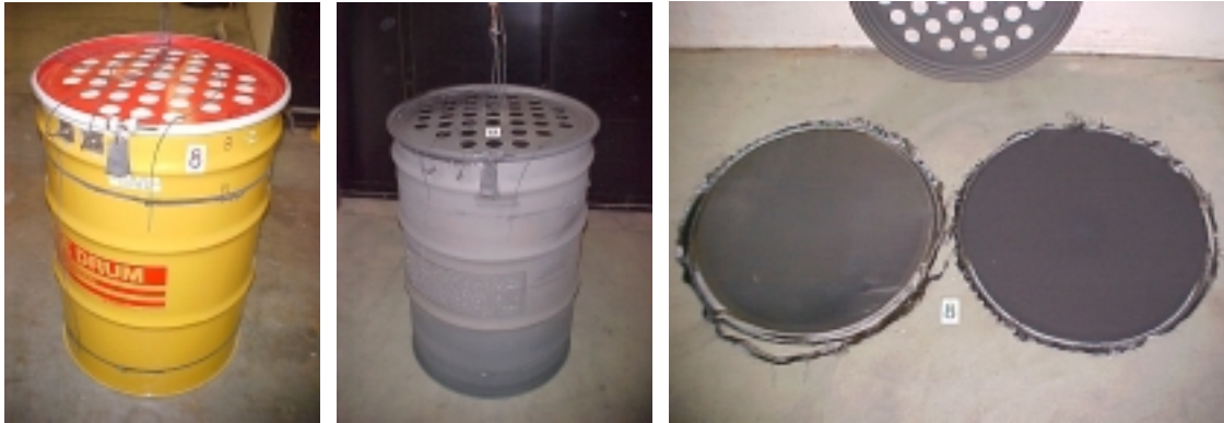
Figure 51. Drum #8 Ready for Pyrolysis
