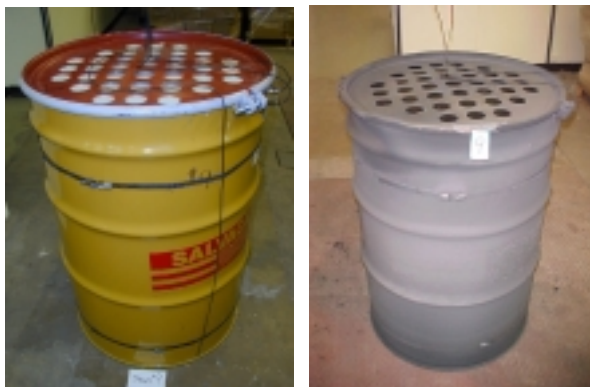
Figure 58. Drum #9 Ready for Pyrolysis Figure 59. Drum #9 Following Pyrolysis
