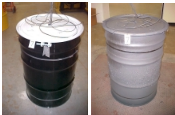
Figure 42. Drum #7 Ready for Pyrolysis Figure 43. Drum #7 Following Pyrolysis
