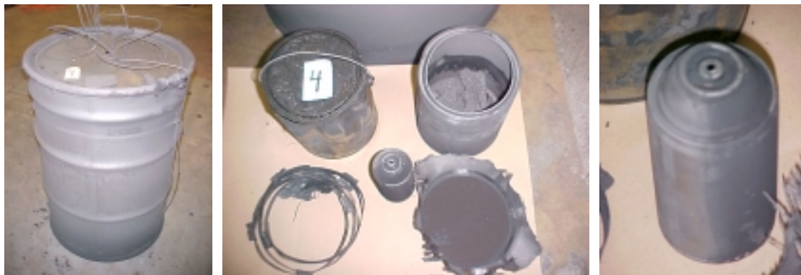
Figure 25. Drum #4 Following Pyrolysis
