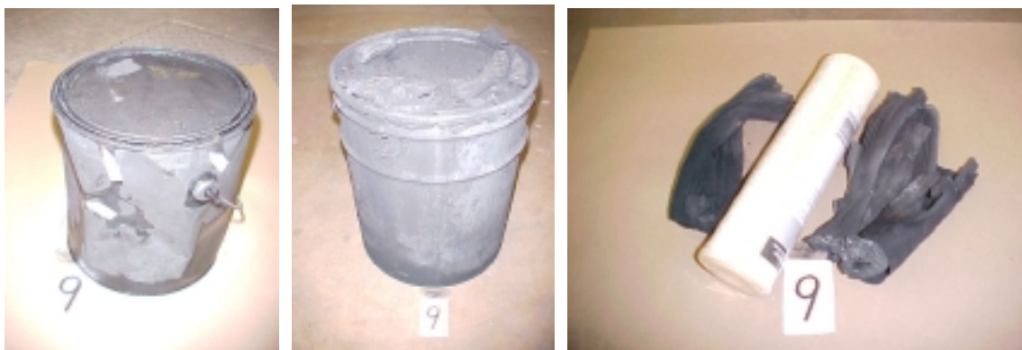
Figure 63. 1-Gallon Can from Drum #9 Following Pyrolysis
