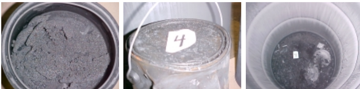
Figure 28. 1-Gallon Can of Anion Exchange Resin from Drum #4 Following Pyrolysis
