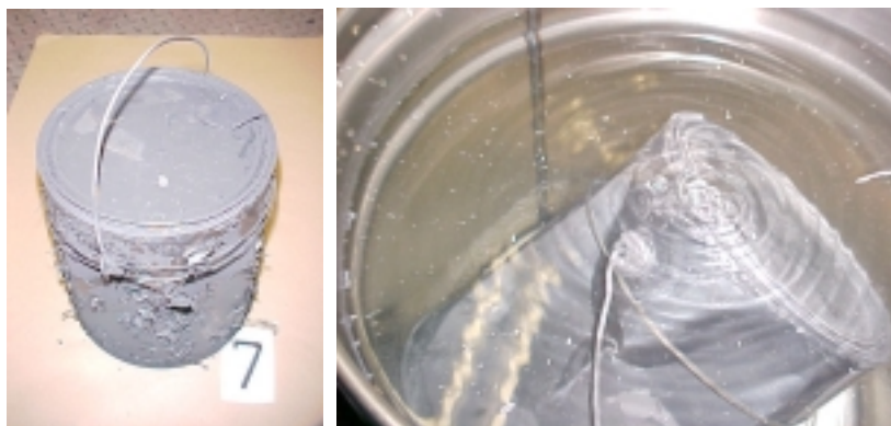
Figure 47. 1-Gallon Paint Can from Drum #7 Following Pyrolysis Figure 48. 1-Gallon Can from Drum #7 During Post-Pyrolysis Leak Testing
