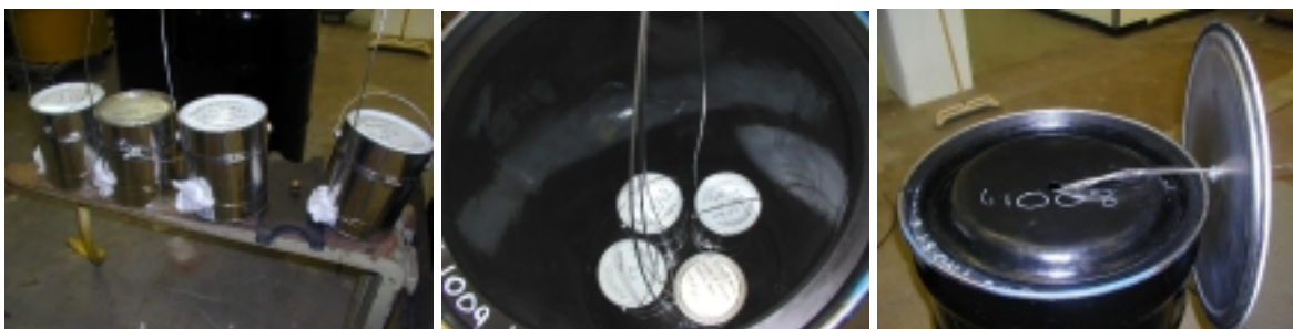
Figure 11. Four One-Gallon Paint Cans for Drum #2 Prior to Pyrolysis, Showing Thermocouple Attachment
