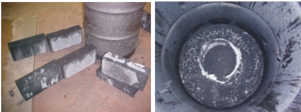
Figure 40. Concrete Blocks from Drum #6 Following Pyrolysis
