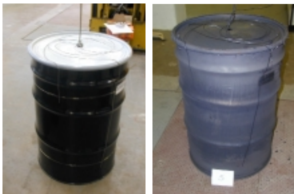
Figure 31. Drum #5 Ready for Pyrolysis Figure 32. Drum #5 Following Pyrolysis
