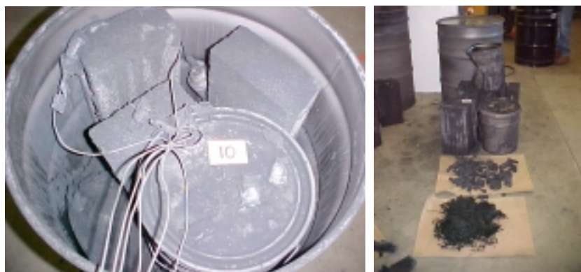
Figure 68. The Interior of Drum #10 Following Pyrolysis Figure 69. The Contents of Drum#10 Following Pyrolysis
