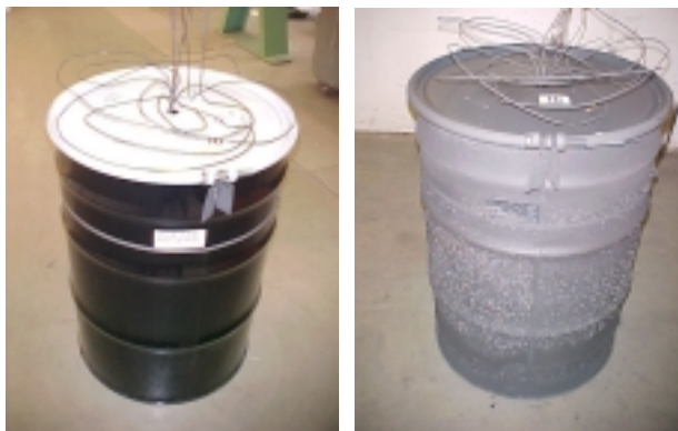
Figure 66. Drum #10 Ready for Pyrolysis Figure 67. Drum #10 Following Pyrolysis
